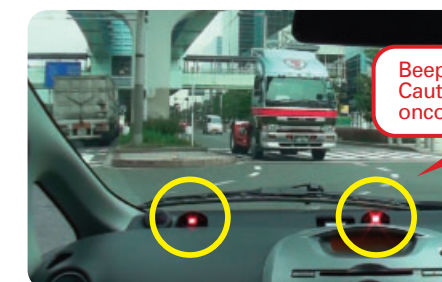
System installed in the i minicar. Without using a car navigation system, it warns the driver with a voice alert and warning light.
